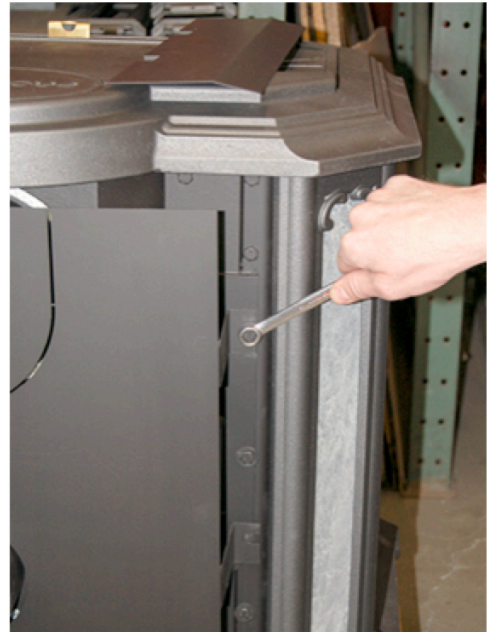
Reinstall hardware to secure center shield (1/2” on top & 5/8” on bottom)
