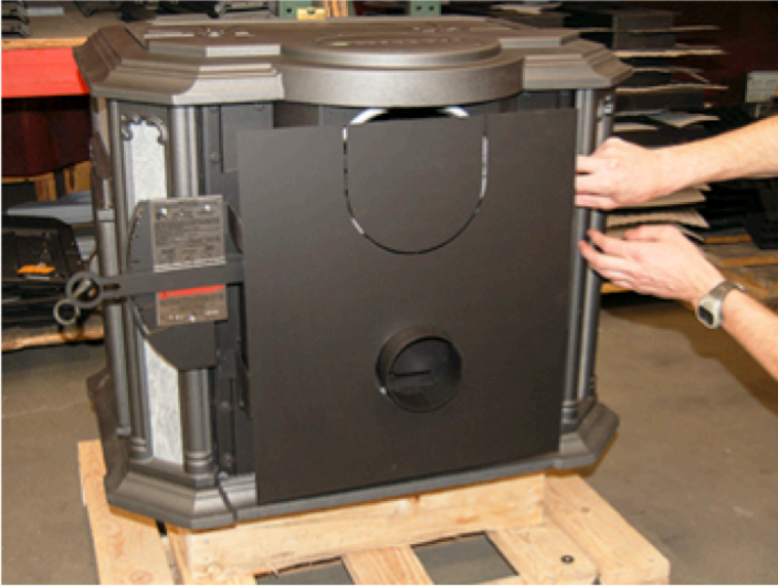
Place center panel over the air intake
