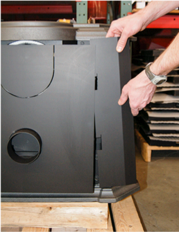
Slide first side panel down into position
